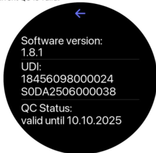
In case you need to do QC procedure you can additionally purchase a QC cartridge. The procedure is exactly the same as the normal measurement process of the device, after which you will see the result of the successful/unsuccessful procedure. In case of successful QC, the expiry date in the menu will be shifted one year forward from the date of the procedure.
